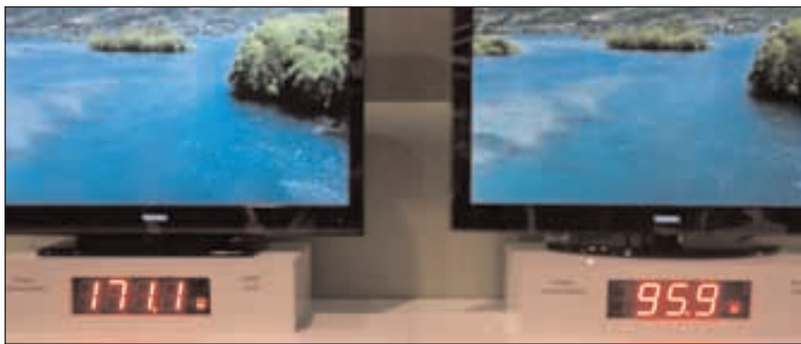
Sharp used this exhibit to illustrate how much more efficient the new LED-backlit LCD TV is versus last year's CCFL equivalent model (the one on the right is marked "2010 LED," while "2009 LCD" is on the left as you look at the photo). At 96 watts, the LED requires little over half as much power as its predecessor while delivering a richer picture evincing especially vibrant greens (if with somewhat darker highlights).
